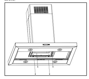
Install the grease filter and turn power on at service panel. Check operation of the hood.
