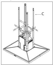
Attach the assembly to the support fixed on the ceiling. Assure with screws (16).
