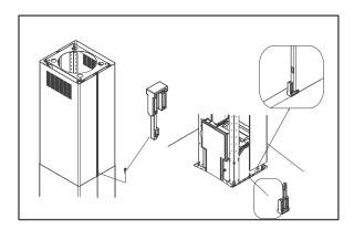
The lower duct cover shall be secured to rangehood by 4 screws.
