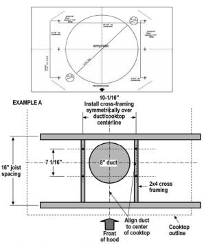
Top view-ceiling joists parallel to front of hood
