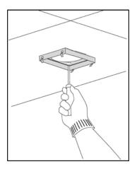
Attach the 4 lower vertical supports (A) to the hood with 16 screws Then attach the lower horizontal support (B) whit 8 screws (inf).
