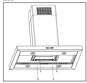
Install the grease filter and turn power on at service panel. Check operation of the hood.
