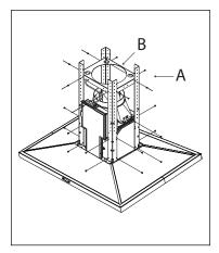
• Attach the 4 upper vertical supports (sup) (c) whit 16 screws to adjust he desired distance.
