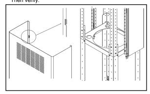
Place lower duct covers using one plastic bracket at each vertex (4 needed).
