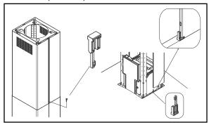
The lower duct cover shall be secured to rangehood by 4 screws.
